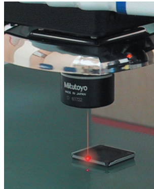
Koaxialer Laser Tracking Auto Fokus (TAF)
